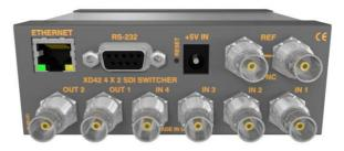
The MSC-XD42L SDI routing switcher has 4 inputs and 2 outputs, supports reclocking of standard 3G/HD/SD SDI rates, automatic bypass of non-standard rates between 20 Mbit/s and 3 Gbit/s, and passes all SDI embedded audio/ancillary data. In addition any output can be independently muted. Switch on vertical sync is provided with the sync reference input with a pass-through connector and provides support for Tri-level sync and NTSC/PAL black burst signals.
